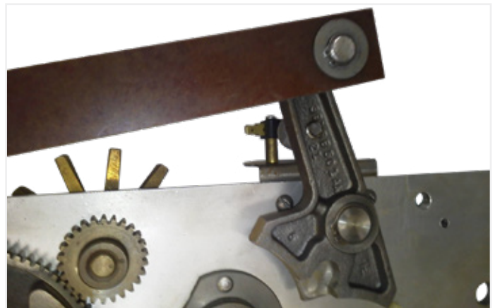
Mechanical stop per C57.131
