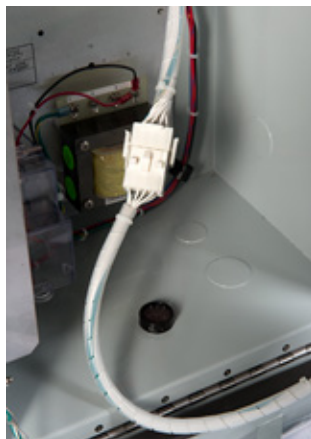
Module to NN Terminal Connector, RC Transformer
